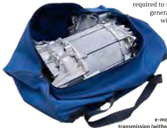
Extremely compact: e-motor with single-speed transmission (without power electronics).
