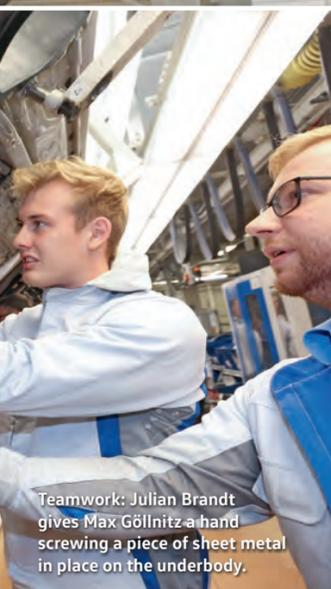
Teamwork: Julian Brandt gives Max Göllnitz a hand screwing a piece of sheet metal in place on the underbody.
